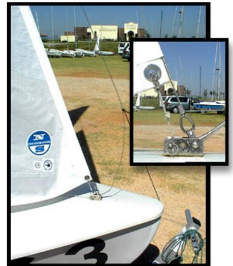
Figure 2 – Jib tack location all the way forward
